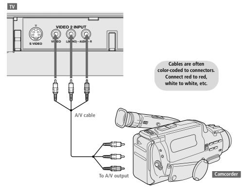
If you have a mono camcorder, connect its audio output jack to the TV's L MONO audio jack.
